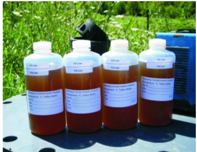
Sample bottles like these filled with leachate were analyzed for contaminants of emerging concern (CECs) including pharmaceuticals, industrial chemicals, household chemicals, steroid hormones, and plant/animal sterols. Photo Credit: Dana W. Kolpin, USGS
