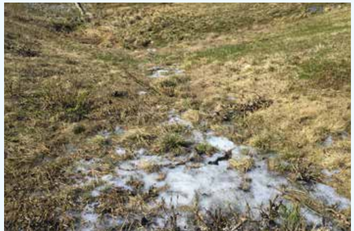
The field team took two grab surface soil samples where they observed foam in a grassy area and in the drainage ditch “to determine if the foam contained PFAS” (AFCEC, 2018b, Section 3, p. 7). Results indicate that the foam used had 12 different PFAS compounds, with PFOS concentrations the highest, at 50 times greater than DEC Soil Migration to Groundwater levels. Photo: Aerostar SES, LLC
